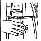
1) Push the release button on the dust cover as shown, and pull it forward
